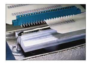
Flow Wells match the component lead pattern and determine the size, shape and direction of the solder flow. Custom Flow Wells can be made up to 15" long and have multiple process sites.
